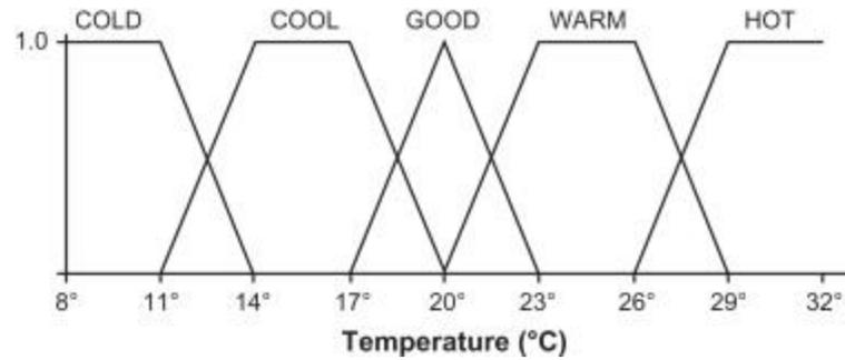
Consider a simplified implementation of an air-conditioning system with a temperature sensor. The temperature might be read by a microprocessor that has a fuzzy algorithm that processes output to continuously control the speed of a motor which keeps the room at a “good temperature”; it also can direct a vent upward or downward as necessary. Figure 7.18 illustrates the process of fuzzification of the air temperature.
